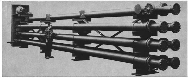
For use in: Vegetable oil fractionations, winterizations of marine and animal oils, separation of tall oil fatty acids, tallow fatty acids, and processing viscous and fouling fluids.
